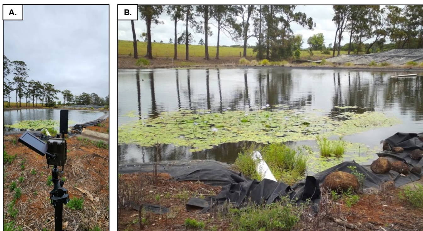
Figure 9. Example of a photo point monitoring setup at a production nursery showing A) Camera trap fitted with solar panels overlooking a water storage, and B) A photo taken by the camera trap of the water storage.
